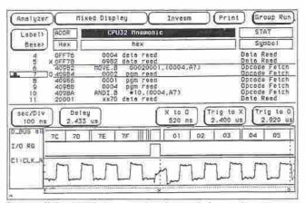
Debug efficiently with time-correlated state, timing, and scope measurements on a single screen.
