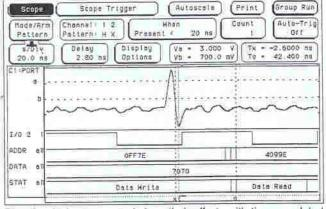
Pinpoint design errors and show their effects with time-correlated scope and timing waveforms.
